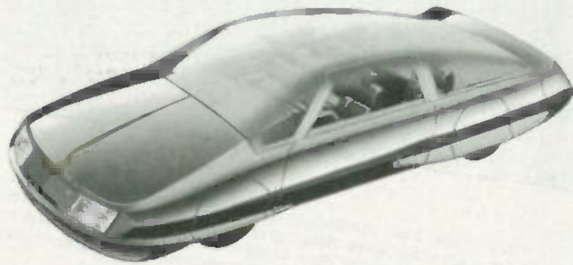
THE ALL-GLASS TDP OF FORD'S 2001 MODEL is flush with the body, giving the car excellent aerodynamic performance.
