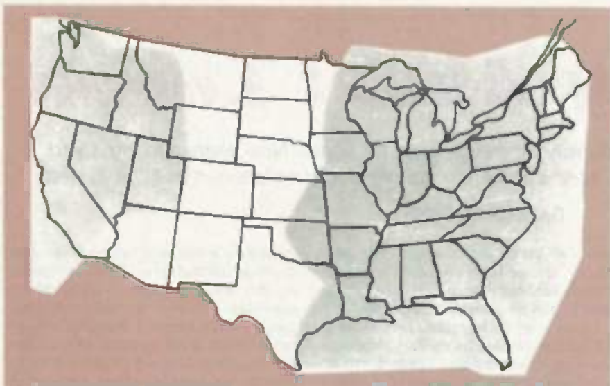
FIG. 1—USABLE LORAN SIGNALS cover much of the contiguous U.S., but a broad area in the midwest is outside the coverage provided by the coastal and Great Lakes chains.
