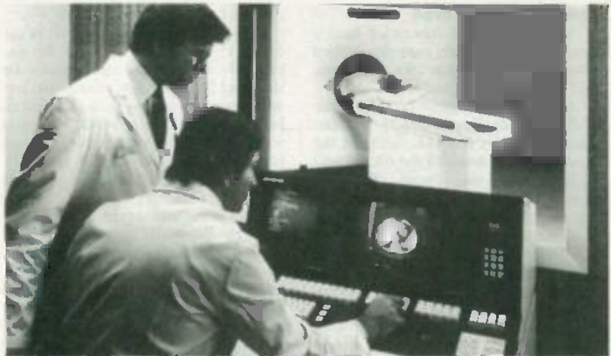
A COMPUTERIZED TOMOGRAPHY SCANNING system combines an advanced X-ray scanning system with a powerful computer to allow doctors to study almost any structure within the human body. Its use often permits patients to avoid exploratory surgery or other painful diagnostic techniques.
